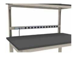
Our standard electrical strip can come as 15 or 20 amperes, 125 volts with an on/off switch, circuit breaker, power indicator light and a 6' power cord. Color is grey. Steel mounting rail is included and is adjustable on our vertical uprights.
